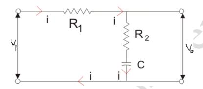
Vi= input from signal generator, Vo= output
