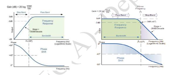
Fig. 1Frequency response of RC (High pass) Fig 2 Frequency response of RC(low pass)
