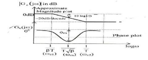
Measurement of Phase Angle:
