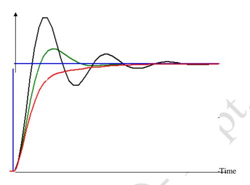
**Result:** Temperature of oven is controlled by using PID controller. By varying P,I,D values two graphs of temperature vs time is plotted.
