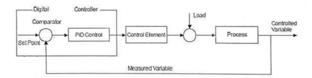
A special case of proportional control is On-off control. If the proportional band of the controller is made very low (=0) the controller output will move from one extreme position to other for slight deviation of process value from the set point. This very sensitive action is called On-off control because final control element is either open (on) or close (off) i.e. operates like a switch. There are the simplest controllers.
